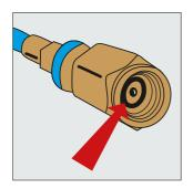
4. If there is a hissing noise, check that the 0-ring is not cracked or dislocated. You can turn this over and refit
