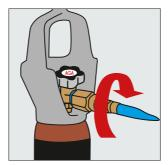
2. Attach the nozzle for the helium by hand. The nozzle can be obtained from your AGA agent.
