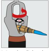
3. Open the cylinder valve slowly until you hear a "puff". If you hear a hissing noise, close the valve and check that the nozzle is securely fitted.
